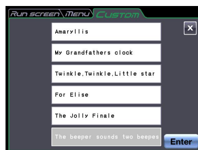
Fig. 2-6-3 (2) Stop signal Setting screen
